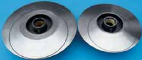
Larger-diameter rotor pulley Previous rotor pulley
