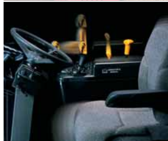
The right-hand console adjusts to fit any operator. In addition, the steering column pivots both at the wheel and at the floor.
