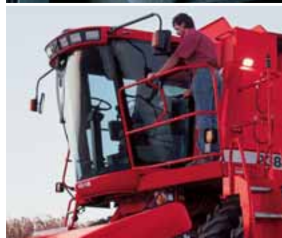
New delayed exit lighting will remain illuminated for 30 seconds after the field lighting switch is turned off for improved night-time exit.
