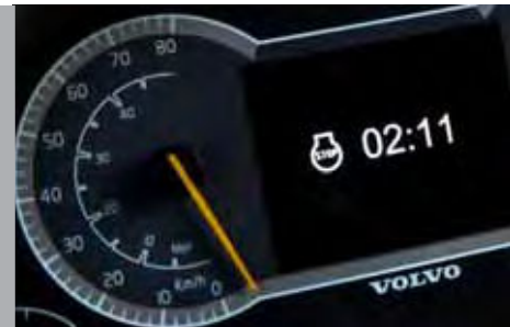
Engine shutdown timer
